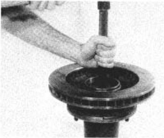
Figure 50 1019-50 Assemble inner wheel bearing cup. Tools: #D-256 Installer, #C-4171 Handle.
