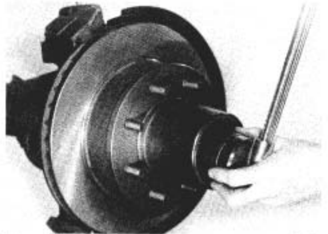
Figure 53 1019-53 To adjust wheel bearings, torque inner adjusting nut to 50 Lb. Ft. (68 N·m) to seat bearings. Rotate hub, then back off inner adjusting nut one-fourth turn maximum. Assemble lock washer, turn nut to nearest hole in washer. Assemble outer locknut and torque to 50 Lb. Ft. (68 N·m). Final bearings adjustment to be .001-.010 (.03-.25 mm) total end play.
