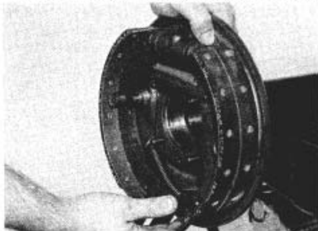
Figure 93 1019-93 Assemble backing plate bolts and backing plate assembly.
