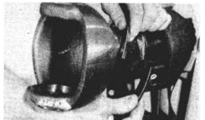
Figure 33 1019-33 Assemble new oil seal with the metal part of the seal towards the end of the axle. Spread split of seal just enough to slip over the tube of the axle.
