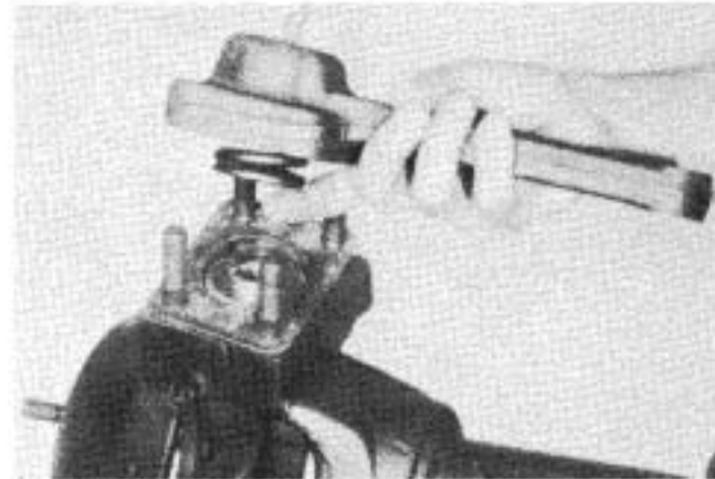
Figure 57 1019-57 Remove steering arm, compression spring, and gasket. Discard gasket, replace with new one at time of assembly.
