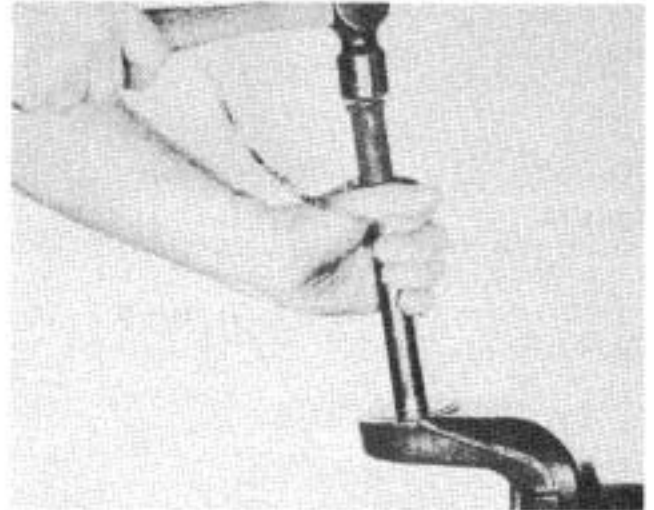
Figure 62 1019-62 Assemble new grease retainer and king pin bearing cup. Tools: #D-142 Installer, #C-4171 Handle.
